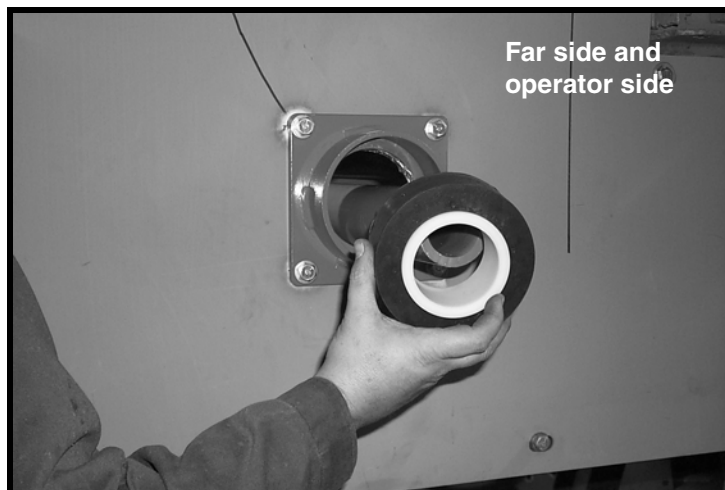
Figure 5. Installing Shock Rings
